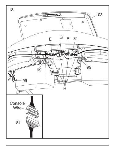
Insert the Console Base Back (93) into the hole in the console assembly and onto the top of the indicated bracket. Be careful not to pinch any wires.
